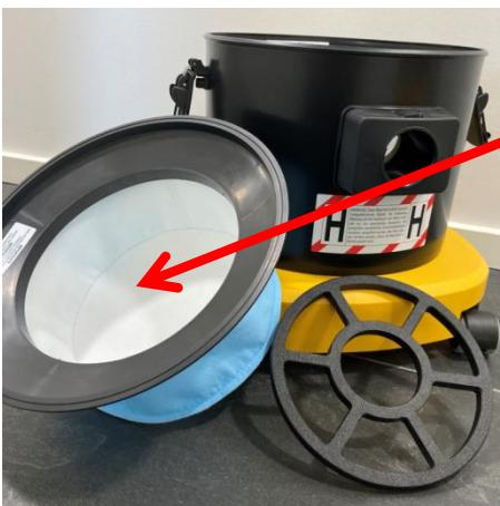
The pre-filter is placed right below the HEPA filter and will protect the HEPA filter in case of a leak in the collection bag.
