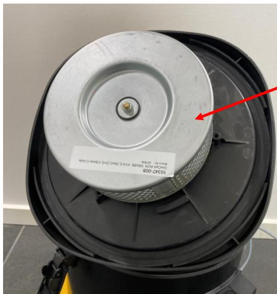
Loosen the two container clips of the motor top and remove the motor top. Place the motor top so that the filter is easily accessible.
