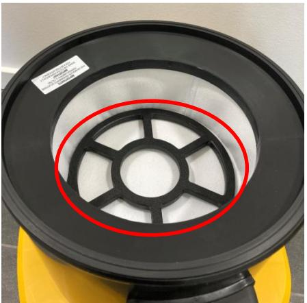
The spacing ring keeps the pre-filter stretched so that it is not sucked closely around the HEPA filter.
